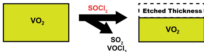
Figure 3. Spontaneous etching of VO 2 by SOCl 2 to produce VOCl 3 and SO 2 as volatile etch products.
