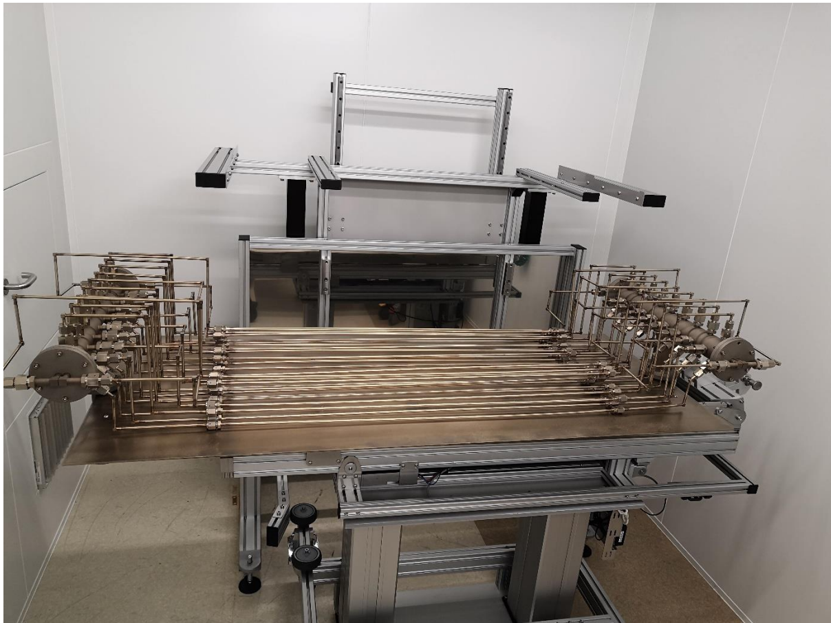
Gas line coating by ALD. Substrate gas lines are fixed at both ends to inlet and outlet manifolds. The setup is loaded in Beneq P800 reactor in place of a reaction chamber for the coating process.
