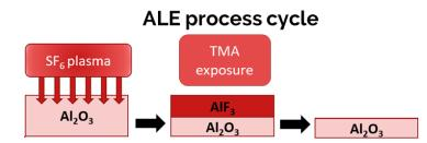
Schematic representation of isotropic plasma ALE of Al<sub>2</sub>O<sub>3</sub> using SF<sub>6</sub> plasma and AlMe<sub>3</sub>. The degree of fluorination affects the required TMA (AlMe<sub>3</sub>) exposure for effective etching.
