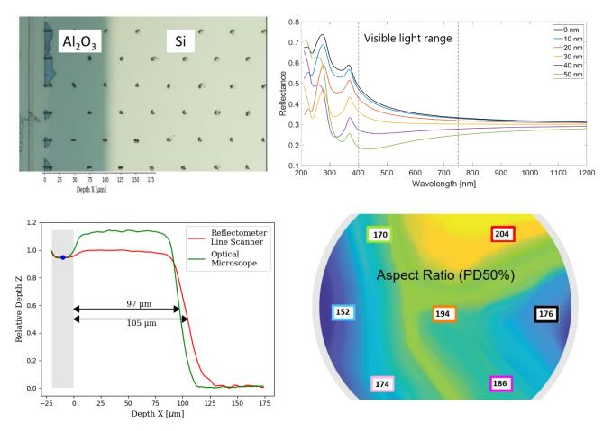
**Figure 1.** Results of ALD Al<sub>2</sub>O<sub>3</sub> (TMA+H<sub>2</sub>O) at 300C, 500 cycles, thickness average 47.2 nm (stdev 0.2 nm over wafer area) deposited onto PillarHall<sup>TM</sup> LHAR test chips placed on the Si carrier wafer.
