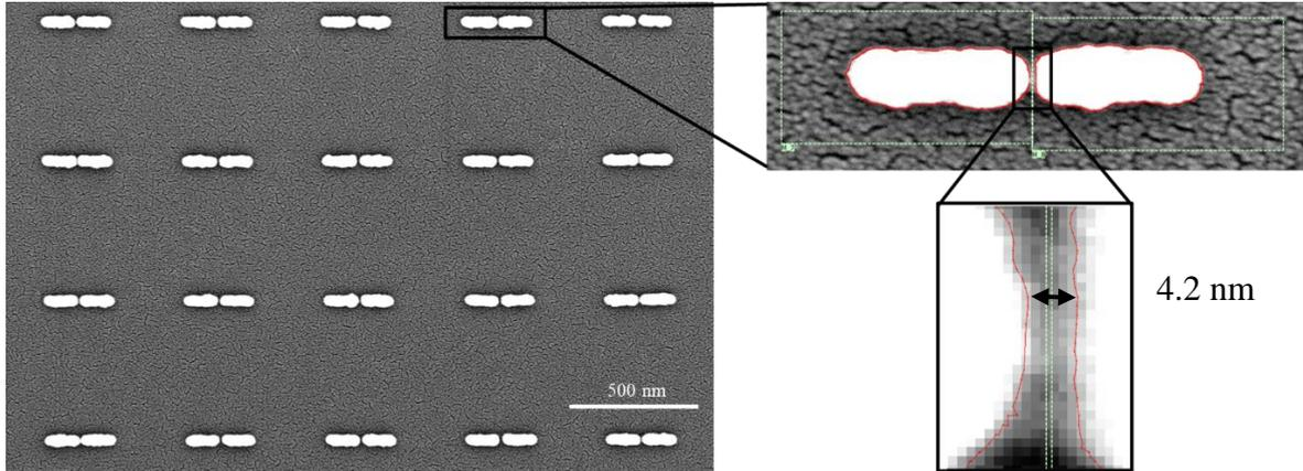
Figure 2. Top down SEM images of arrays of Pd/Au nanoantenna dimers after 200 cycles of Cu AS-ALD at 230 C. A thin Au layer is sputtered onto the quartz substrate for imaging.
