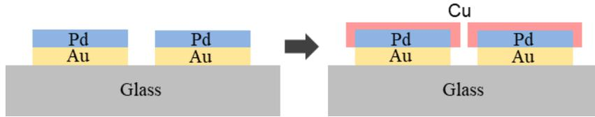
Figure 1. Side view schematic diagram of AS-ALD to tune nanogaps.
