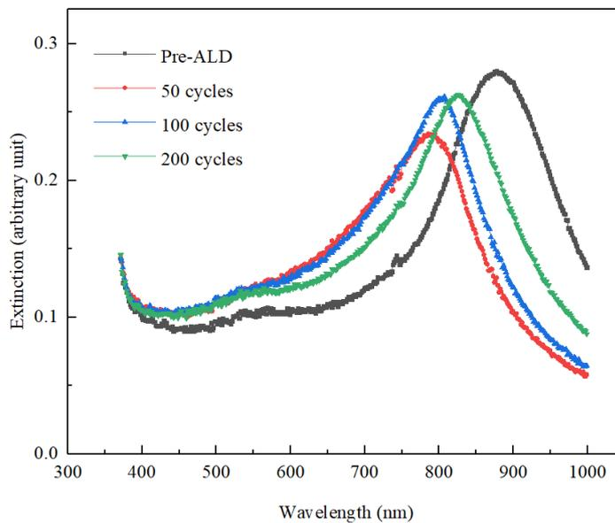
Figure 3. Extinction curves of arrays of Pd/Au nanoantenna dimers in the Cu AS-ALD process.
