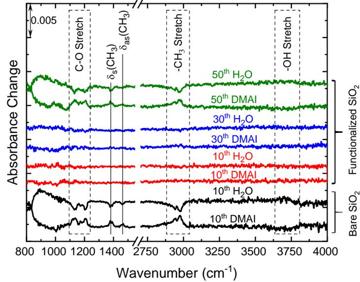
Figure 1. Infrared absorbance change for the DMAI and H<sub>2</sub>O half-cycle during ALD of Al<sub>2</sub>O<sub>3</sub> on bare SiO<sub>2</sub> (10<sup>th</sup> cycle) and functionalized SiO<sub>2</sub> (10<sup>th</sup>, 30<sup>th</sup>, and 50<sup>th</sup> cycles).
