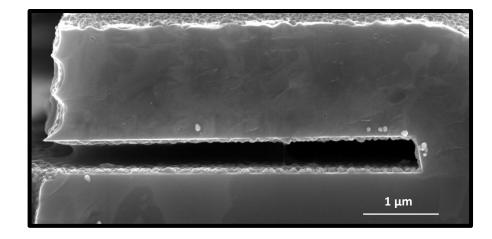
Scanning Electron Micrograph (cross section) of Ag thin film deposited on lateral high aspect ratio structure (10:1) showing the degree of conformality of the film. The scale bar represents 1  $\mu$ m.
