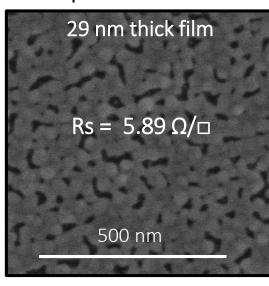
Scanning Electron Micrographs (top view) of Ag thin films (29 nm thick) deposited on glass substrates showing the principle of the two-step processing: product 1 obtained by plasma-enhanced deposition exhibiting a high sheet resistance Rs (left) and product 2 obtained after post-treatment exhibiting a low sheet resistance Rs (right). The scale bars represent 500 nm.
