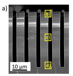
Figure 2. Scanning Electron Microscopy images of  $Ta_2O_5$  thin film formed on 3D structures with AR=13 by Plasma Enhanced Atomic Layer Deposition followed by postgrowth wet etch. a) A general view and detailed images of as-grown deposit and structure after postgrowth wet etch at b) the top, c) the middle and d) the bottom of the 3D structure. Note the densified film at the first four DRIE-characteristic undulated sidewalls of 3D structure in b).
