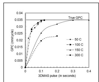
**Fig. 1.** Experimental GPC vs. precursor pulse shows that at 50 °C, 100 °C and 150 °C the self-limiting, surface saturated GPC is achieved. However, at 300 °C a much lower GPC is observed indicating that the reaction is not self-limiting.
