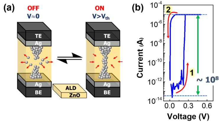
Figure 1. Ag-based threshold switching layer in a selector device. (a) Conceptual sketch showing how filamentary Ag-based threshold switching selector works. (b) DC I-V curve showing ultra-steep threshold characteristics for ALD grown ZnO switching layer.
