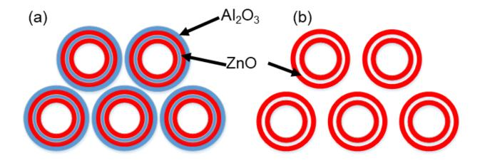
Figure 1. Schematics of ZnO nanotube synthesis method before (a) and after (b) NaOH etching.
