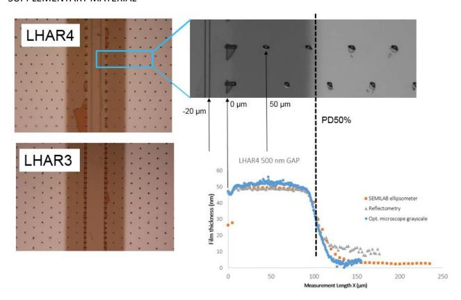
Fig S1. (Left) Microscope images of 50 nm ALD Al2O3 on PillarHall LHAR3 and LHAR4 after removal of the top membrane. LHAR4 has advanced pillar design and internal distance indicator line on the opening area to support optical characterization by imaging and line-scan methods as illustrated in detail in gray-scale image.
