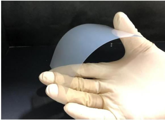
Fig1: Aluminosilicate thin film on a PEN film.
