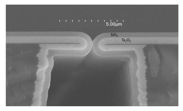
~ 400 nm SiO<sub>2</sub> deposited at 180 cycles per minute on trench with overhanging aperture. ~500 nm of  $Ta_2O_5$  was previously deposited using conventional pulsed ALD, to provide image contrast and narrow aperture.
