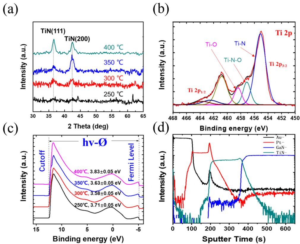
**Figure.** (a) XRD patterns TiN films deposited at different temperatures; (b) High resolution XPS spectra of Ti 2p orbital in TiN films deposited at 350 °C. Binding energy was calibrated with C-C peaks; (c) UPS measurement of TiN films deposited at different temperatures with -5 bias voltage applied on the sample; (d) *n*-GaN/TiN(50nm)/Pt(50nm)/Au(100nm) sample annealed at 700 °C in N<sub>2</sub> for 1 min ToF-SIMS depth profile.
