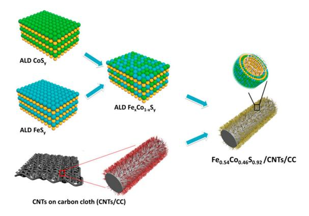
**Scheme 1.** Schematic illustration of the ALD-based bottom-up engineering strategy for an electrocatalyst. The strategy involves two separate optimization steps, i.e., the compositional optimization of ternary  $Fe_xCo_{1-x}S_y$  by ALD for high specific activity and the geometric optimization of the electrode structure via nanostructuring for high surface area.
