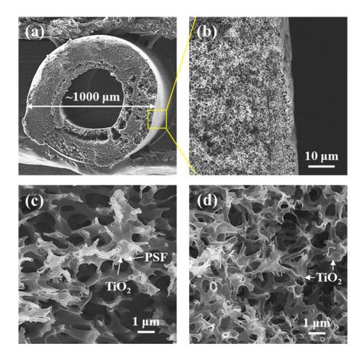
**Figure S1.** SEM images of (a) PSF hollow fiber and (b) its outer wall in the inset of (a). TiO<sub>2</sub> interconnected nanotubes in the hollow fibers before (c) and after (d) the removal of PSF by annealing at 500 °C.
