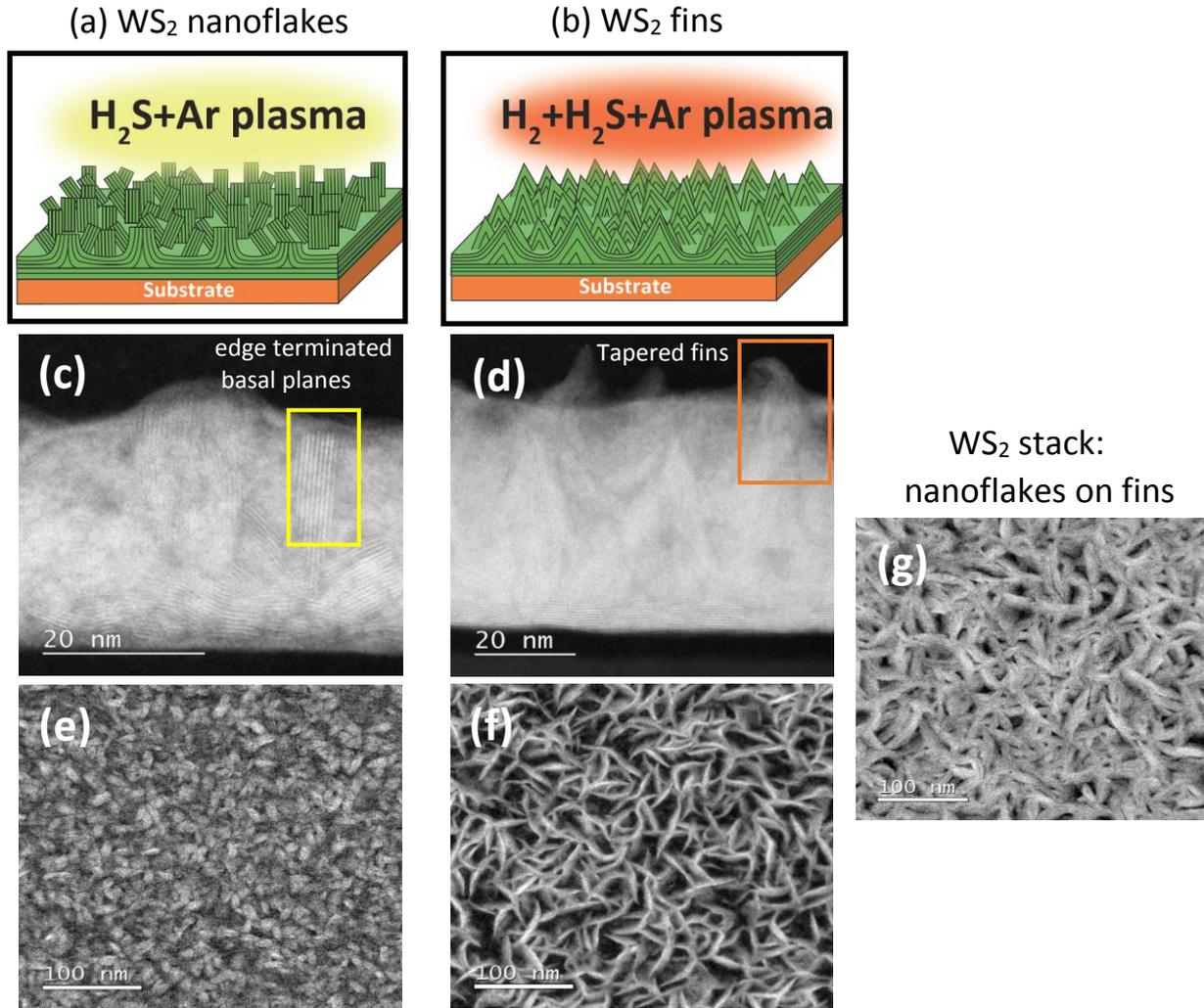
Fig.1. (a, b) Scheme for the WS<sub>2</sub> nanoflakes and WS<sub>2</sub> fin growth. (c, d) Cross-section transmission electron microscopy (TEM) images of WS<sub>2</sub> nanoflakes and fins. (e, f, g) Top-view TEM images of WS<sub>2</sub> nanoflakes, fins and stack (nanoflakes on top of fins), respectively.
