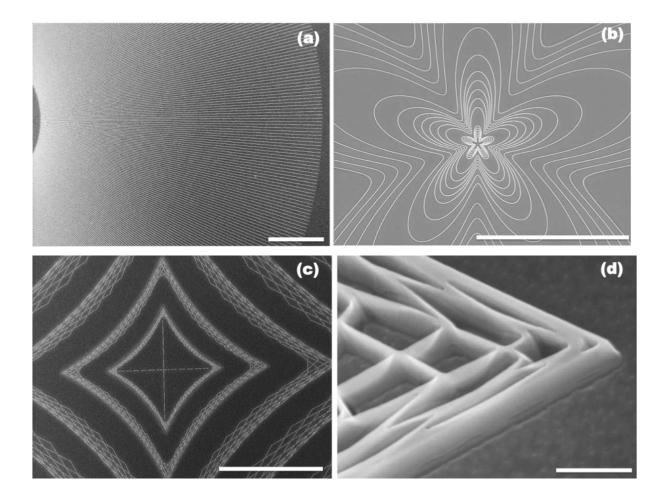
Figure 1. SEM images of nanoscale patterns with different geometries and feature sizes fabricated with electron beam lithography: (a) radial lines with gap size up to 1000 nm with the distance between two neighboring lines changing by 10 nm within 1  $\mu$ m; math defined lines with (b) different curvatures and (c, d) different intersection angles. (d) SEM image taken at 30° tilt after the ALE process: 200 nm deep etching, 850 cycles. The scale bars are 30  $\mu$ m (a, b, c) and 500 nm (d).
