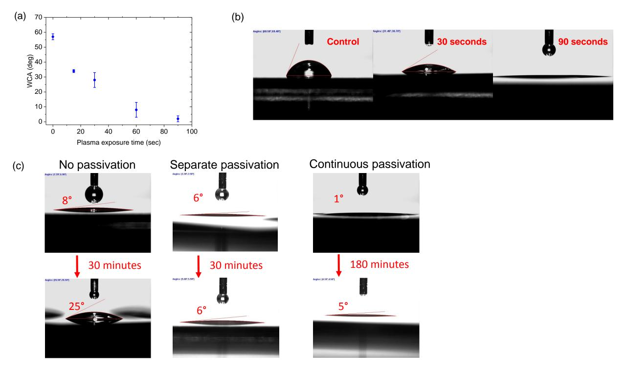
Abstract Figure. (a) Water contact angle (WCA) as a function of plasma exposure time. (b) Water droplet shape evolution with increasing plasma exposure time. (c) Water droplet size before (top row) and after (bottom row) ambient clean room exposure.
