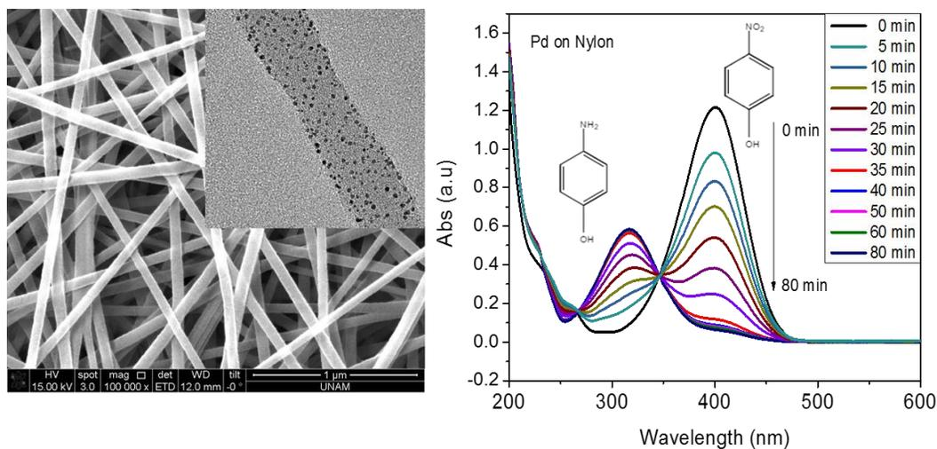
**Figure 1.** SEM and TEM as inset for ALD of Pd nanograins on polymeric nanofibers (left) and its effective catalytic properties (right)
