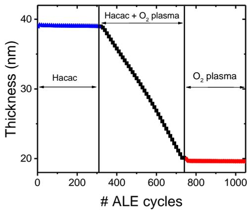
**Figure 1:** ZnO thickness as a function of the number of plasma-assisted ALE cycles. From left to right alternating pulses of: Hacac and O<sub>2</sub> gas (blue), Hacac and O<sub>2</sub> plasma (black) and only O<sub>2</sub> plasma (red).
